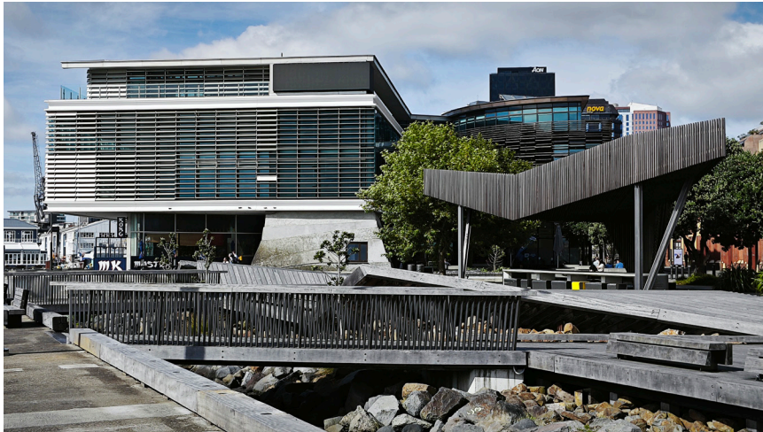
Fig. 2. Continuous timber deck as public ground plane, Wellington waterfront. Board direction indicates the line of movement; the gap module governs drainage and drying rate [photo by the authors, 2026]
