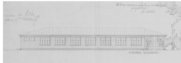
Fig. 9. Design of a standard 28-bed barrack for the teachers' sanatoriums in Jurbarkas and Varėna (civ. eng. Alfonsas Maculevičius, 1939) [Lithuanian Central State Archives, f. 380, ap. 1, b. 1730, l. 89]
