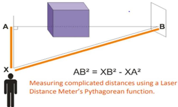
**Figure 2.** Measurement of complex distance with the laser rangefinder method (source: [www.transcat.com](http://www.transcat.com))
