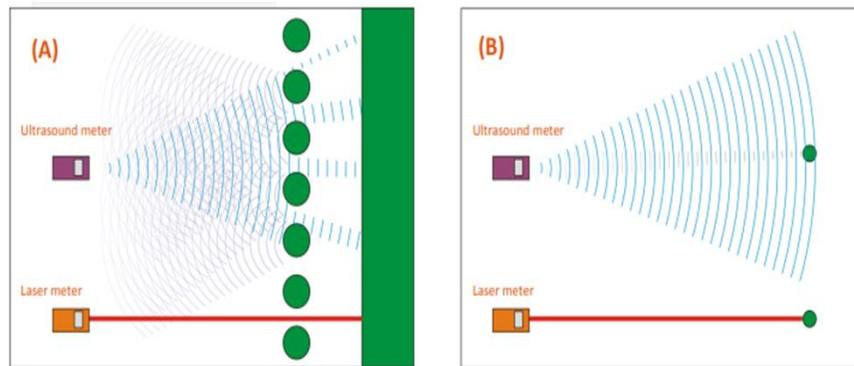
**Figure 3.** Limitations on the use of ultrasonic rangefinders (source: [www.transcat.com](http://www.transcat.com))
